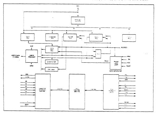
Figure 2. WD279X BLOCK DIAGRAM
