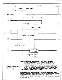
FIGURE 3. READ ENABLE TIMING
