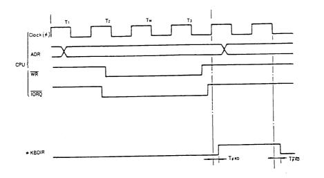
Note 13: The signal marked with an asterisk is the KBDIR output of MA18 when "1" is applied to the  $\overline{X5}$  during reset.
