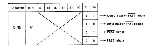
The PRST signal can be generated by the external circuit.
