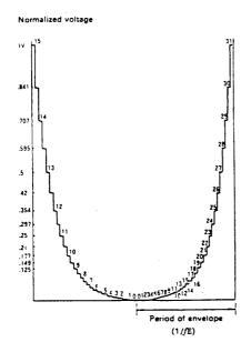
Fig. 1 Output level of DA convertor The subscripts on the left half of the diagram are the fixed levels of the selection signals L<sub>3</sub>, L<sub>2</sub>, L<sub>1</sub>, and L<sub>0</sub> converted into decimal values. The subscripts on the right side are decimal expressions of the envelope counter output signals E<sub>4</sub>, E<sub>3</sub>, E<sub>2</sub>, E<sub>1</sub>, and E<sub>0</sub>.
