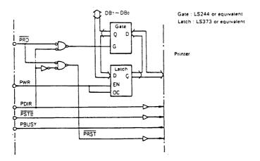
PBUSY: If a signal is input to the PBUSY pin and read, the same level as input to B1 is output.
