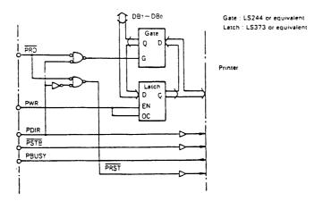
PBUSY: If a signal is input to the PBUSY pin and read, the same level as input to B1 is output.
