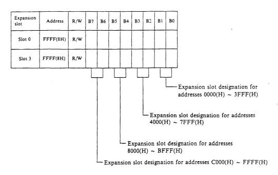
The slot expansion function is controlled by the level of the  $\overline{X1}$  and  $\overline{X3}$  pins when the device is reset. Refer to section on selection of this function.
