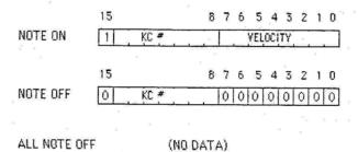
KC#(Keycode number) indicates an 8-octave range, with the note name being represented by the lower 4 bits, and the octave by the upper 3 bits. This KC# format is internal to SFG-05 as shown in the following.
