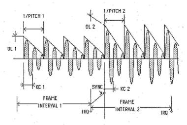
The above illustrates the principle of CSM voice synthesis. That is, one spectrum component of possible four formants is generated. Within the frame interval, exponentially decaying sin-wave ( with its formant frequency and intensity being KC and OL respectively) is repeatedly calculated with the given pitch.
