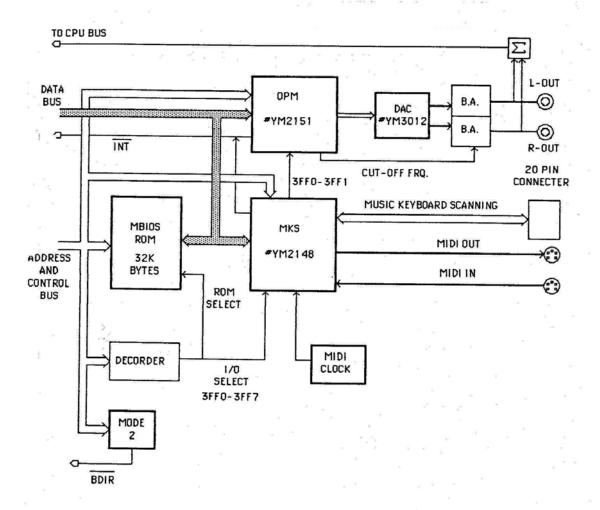
FIG. 1.2. HARDWARE CONFIGURATION OF SFG-05
